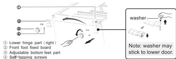
9. Screw out lower hinge, change it to the near hole site, and then screw up and mount washer.
