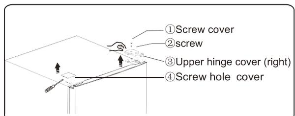
3. Unscrew the flange screws ① which are used for fixing the right upper hinge part ②. Lift the upper door and place it on a padded surface to prevent it from scratching.
