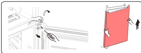
6. Place the lower door on a smooth surface with its panel upwards. Loose screws ②, detach part ①. Then install part ① to corresponding position on left side together with screws ②.
