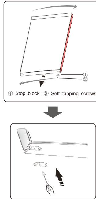
7. Change screw hole covers on middle cover plate from left to right (as shown in figure below).
