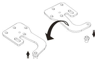
13. Just remount to the step 2, change upper hinge cover③to left and fix them with screws② and then install the screw cover①. Finally, change screw hole cover④to right.
