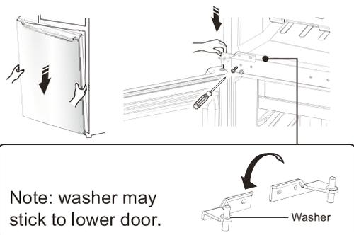
12. Screw out The upper hinge axis, turn the upper hinge over and fix axis on it. Then place it at side for use.
