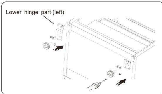
11. Move the lower door and adjust its position to align lower hole site and upper hinge axis. Turn the middle hinge by 180, change the washer on the axis to the upper side, adjust the middle hinge to the appropriate position and then install it.
