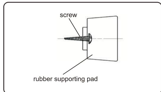
3. Make screw in alignment with the hole on lower base cover. Fasten rubber supporting pad to the base cover firmly by a cross screwdriver (self-provided).
