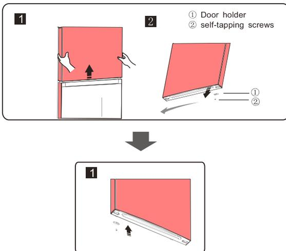
5. Loose screws used to fix the middle hinge and remove middle hinge. Then remove the lower door.
